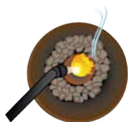
Mercury/gold amalgam heated to evaporate Hg
